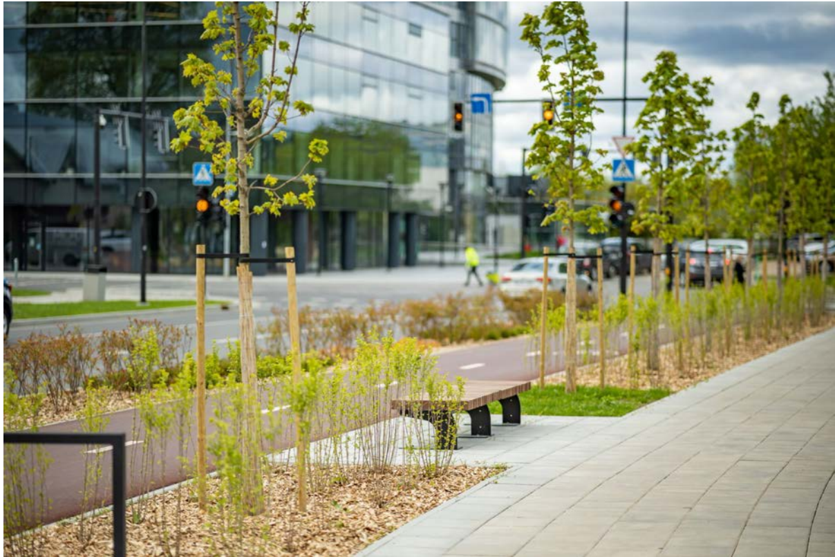
Picture 7. 3 Vilnius Street design example, with three sections for cars, bicycles and pedestrians separated by green infrastructure.
