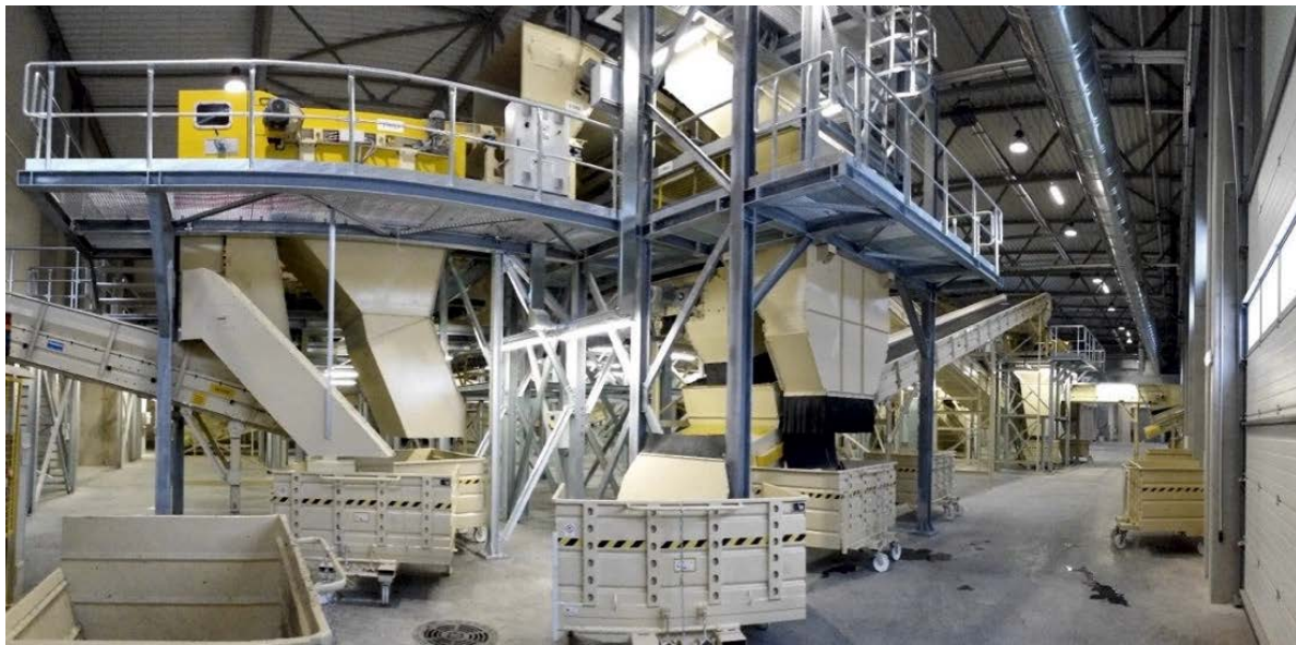
Graphic 4. 2 Modern mechanical-biological waste treatment facilities operated by Vilnius Region Waste Management Center.
